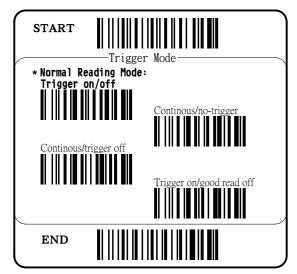
Normal Reading Pushing the keytop, the LED is keeping on. Off the keytop or Mode: Trigger while the scanner has a good read, the LED is off. When the on/off LED is off by losing the keytop, the LED will be On again while we pushing the keytop again and ready to read decoding code.
